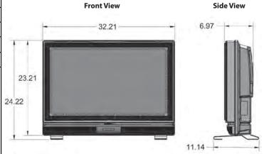
TV Dimensions are: 32.21 in. W x 23.21 in. H x 6.97 in. D Height dimension with table top stand is 24.22 in. Depth dimension with table top stand is 11.14 in.
